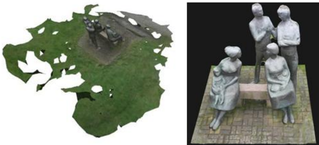
Figure 22. Raw 3D model after automatic photogrammetric rendering (left) being clipped and transformed with 3DEdit to final a 3D model (right).
